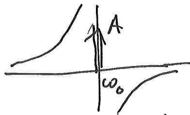
For  $\omega \ll \omega_0$   $\tilde{\chi}'(\omega) \cong \frac{2}{\pi \omega_0} A$  (D.C. polarizability related to lowest absorption resonance)
