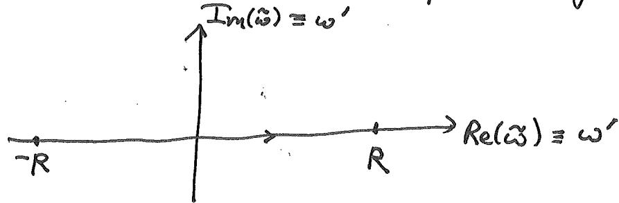
Evaluate integral on  $\text{Re}(\tilde{\omega})$  axis using contour integration.
