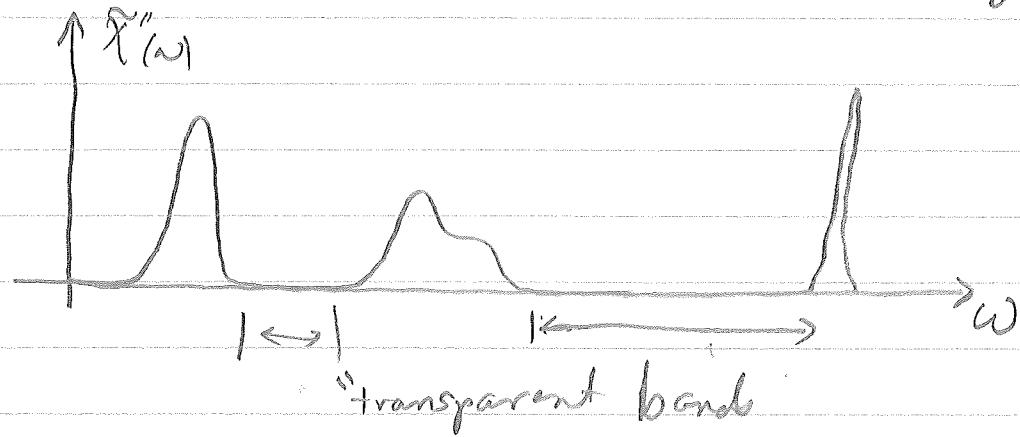
For the range of frequencies for which  $\tilde{\chi}''(\omega) \approx 0$  the medium is transparent, with negligible absorption. In such bands,
