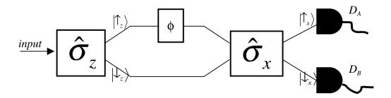
Spin-1/2 electrons are prepared in a given state (pure or mixed) are separated in two paths by a Stern-Gerlach apparatus (gradient field along z). In one path the particle passes through a phase-shifter, which imparts a relative phase  $\phi$ . The two paths are then recombined, sent through another Stern-Gerlach with gradient along x, and the particles are counted in detectors in the two emerging ports.
