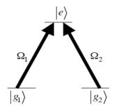
The two ground states are resonantly coupled to the excited state, each with a different Rabi frequency. Taking the two ground states as the zero of energy, then in the RWA (and in the rotating frame) the Hamiltonian is
