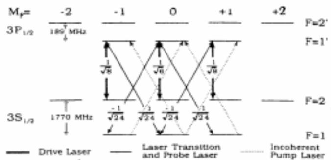
g.2a. Three level  $\Lambda$  atomic system for LWI any state bases.
