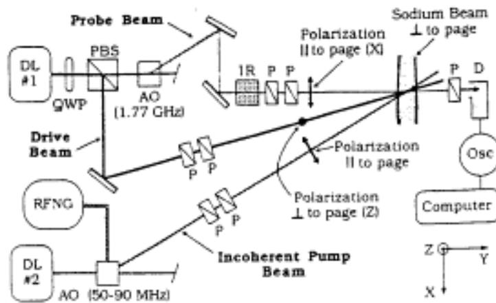
Fig.3. Schematic of the experiment to observe inversionless gain and cw laser oscillation. DL –dye laser, AO – acousto-optic modulator, RFNG – rf noise generator, D – detector.
