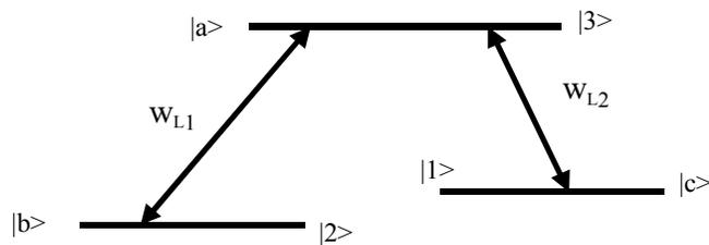
Fig.1.Three-level atom in the  $\Lambda$ - configuration interacting with two fields of frequencies  $w_{L1}$  and  $w_{L2}$ .
