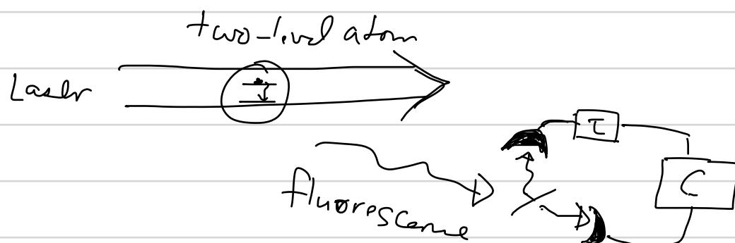
If one photon counter clicks, we immediately measured that the atom jumped to the ground state. It takes time for the atom to be re-excited — the atom near emits two photons of this color at one time  $\Rightarrow$  Photons are never arriving at the same time  $\Rightarrow$  antibunching!
