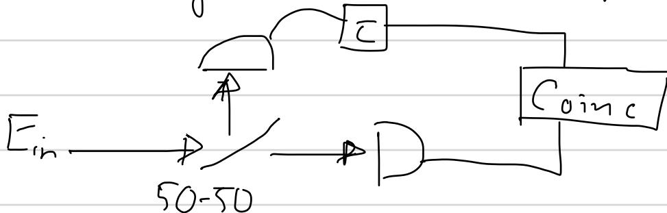
Photons counters, symmetrically placed on opposed output ports of a 50-50 beam spl. br
