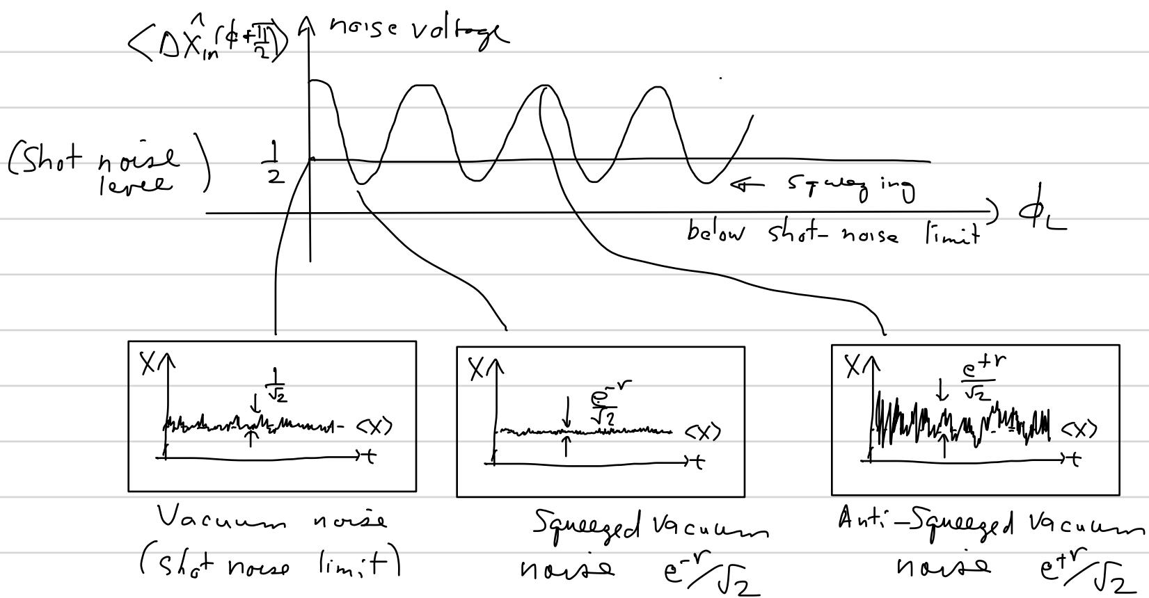
The level of fluctuations seen in the photodetector depends on the phase of local oscillator. Interfering the squeezed vacuum with the coherent state of the local oscillator has reduced the fluctuations beyond the vacuum level, sometimes known as the "standard quantum limit".
