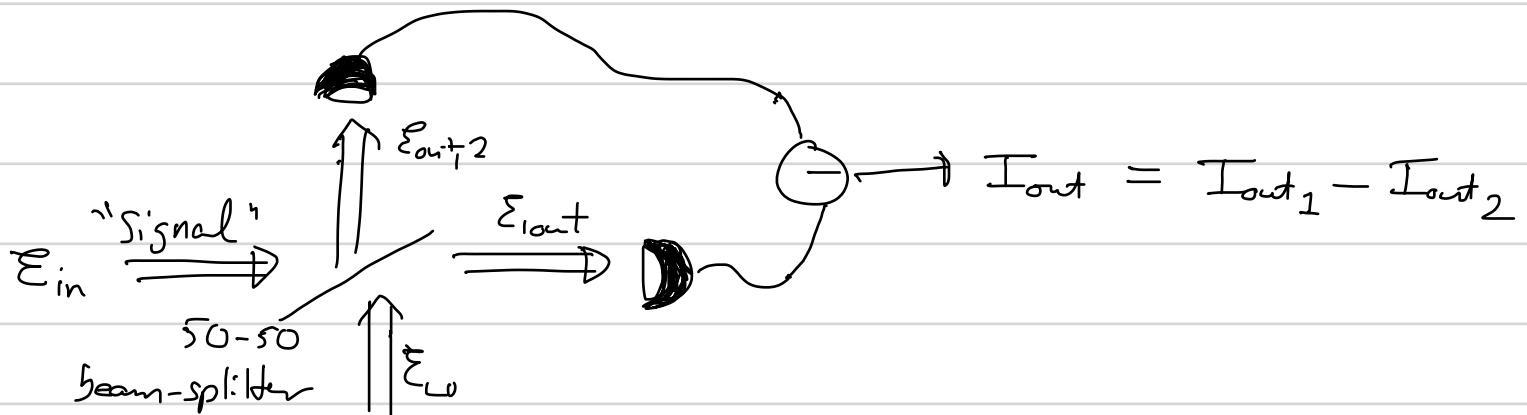
We now detect the field at the two output ports of a 50-50 beam splitter after interfering the signal with the local oscillator. Again assuming a symmetric beam-splitter
