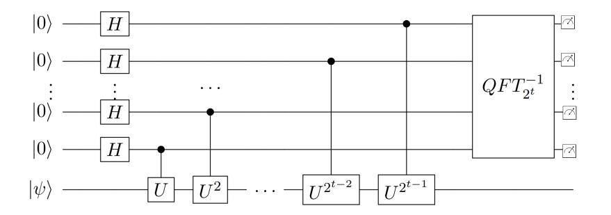
This is the entire phase estimation circuit. The measurements at the end read of the corresponding bits in the binary expansion of  $\theta$ .
