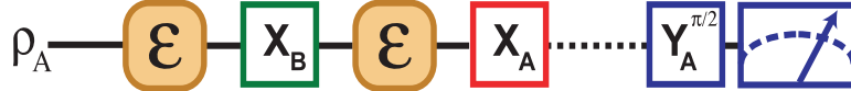
FIG. 3: (Color online) A single ping-pong of the qubit between Alice and Bob in the coherent-transport protocol, with the decohering CPTP map included in the two traverses of the quantum channel.
