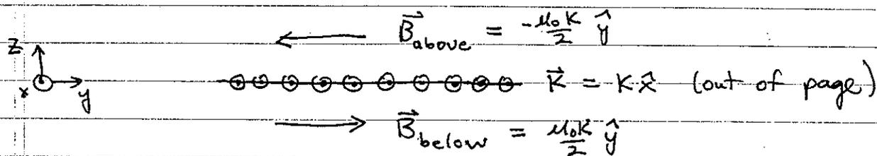
$$\Rightarrow \vec{A}_{\text{above}} = -\frac{1}{2} (\vec{r} \times \vec{B}_{\text{above}}) = -\frac{1}{2} \begin{vmatrix} \hat{x} & \hat{y} & \hat{z} \\ x & y & z \\ 0 & -\frac{\mu_0 K}{2} & 0 \end{vmatrix}$$
