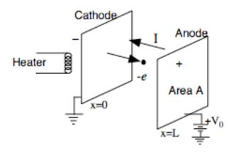
Parallel plate capacitor, Area A, distance L between plates
