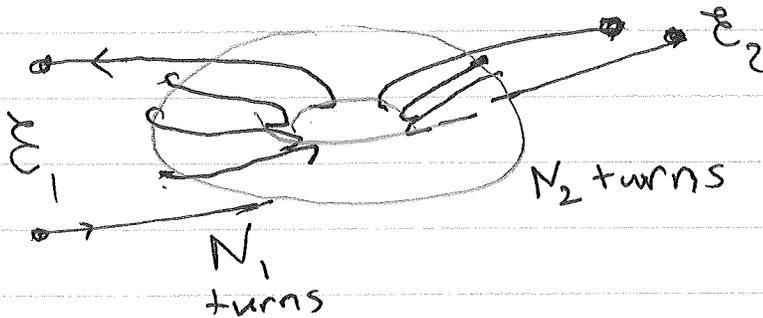
Here I draw the transformer as coils wrapped around an iron ~~plate~~ torus.
