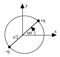
The motion of this dipole can be model by the superposition of two linearly oscillating dipoles that are 90° out of phase with one another:  $\mathbf{p}(t) = p_0 \cos(\omega t) \hat{\mathbf{x}} + p_0 \sin(\omega t) \hat{\mathbf{y}}, \quad p_0 \equiv qs$ .
