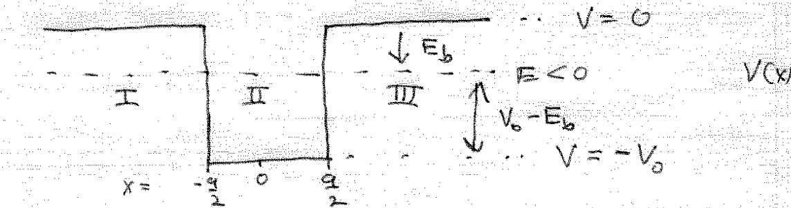
With the zero of potential energy as chosen above, the bound states have  $E < 0$ . The "binding energy" is defined  $E_b = -E$ .
