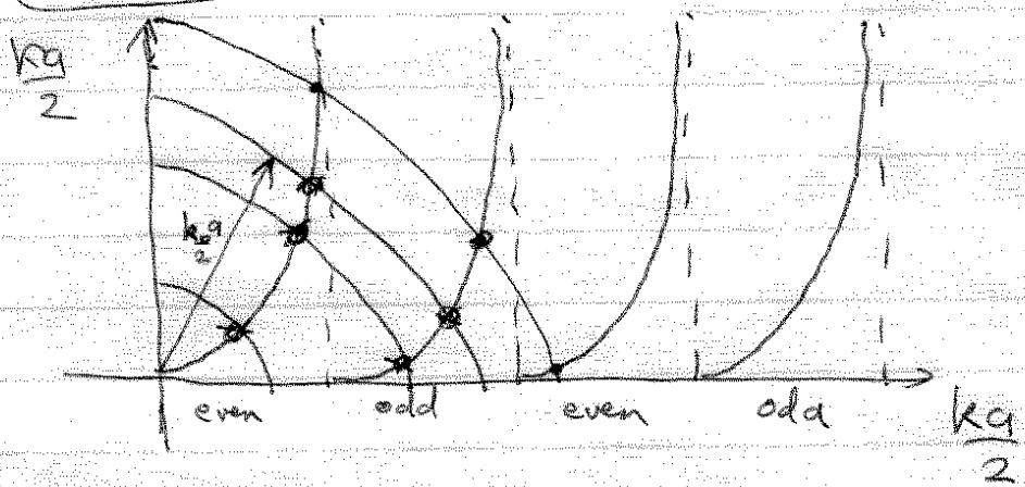
The intersection points represent the solution for a given potential depth  $V_0$ .
