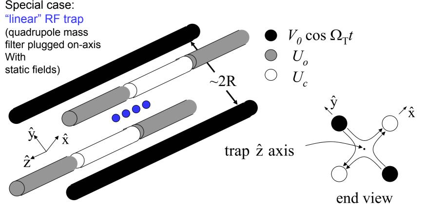
$$\Phi = \frac{(x^2 - y^2)}{2R^2} V_0 \cos \Omega_T t + \frac{(U_x x^2 + U_y y^2 + U_z z^2)}{2R^2}, \quad \sum_{i=x,y,z} U_i = 0$$
