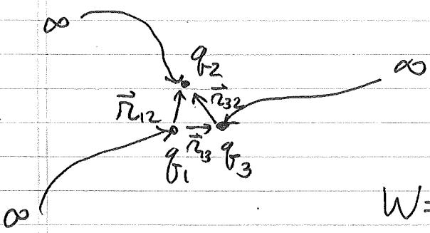
$$W = \frac{q_1 q_2}{r_{12}} + \frac{q_1 q_3}{r_{13}} + \frac{q_2 q_3}{r_{23}}$$
