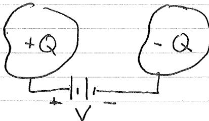
Induced charge purely a function of geometry
