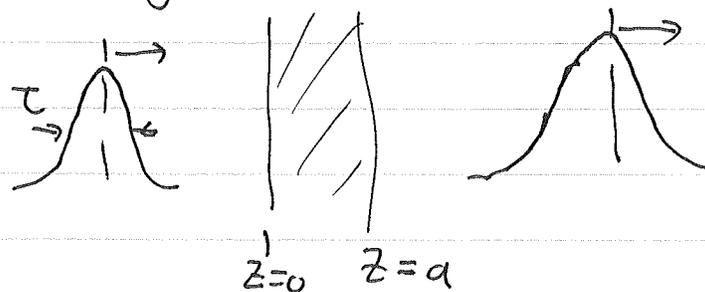
(a)  $z=0 \quad E^{(+)}(t) = E_0 e^{-\frac{t^2}{2\tau^2}} e^{-i\omega_0 t}$  (Gaussian, width  $\tau$ )
