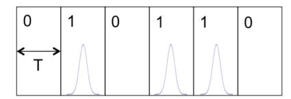
The rate of data transmission (bits/second) is then 1/T. The window is taken in order to avoid overlap. It can be shown that if we can tolerate a bit rate error no greater than  $10^{-9}$ , then the time window must be 2 times the pulse duration. Of course the name of the game is to maximize the bit-rate over the longest possible distances. However, very short pulses have broad spectra, and thus spread very rapidly.
