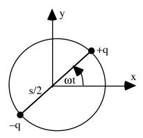
The motion of this dipole can be model by the superposition of two linearly oscillating dipole which are  $90^{\circ}$  out of phase with one another:
