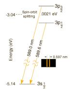
These two lines are known as the "sodium doublet". The transition  $3s_{1/2} \rightarrow 3p_{1/2}$  is known as "D1" and  $3s_{1/2} \rightarrow 3p_{3/2}$  known as "D2". All the alkalis have this basic structure.
