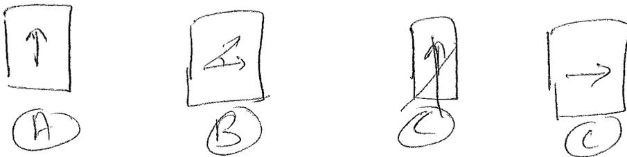
without Polarizer (B), (A) & (C) are orthogonal and nothing passes (C). However by inserting the middle polarizer and maximizing the passage of intensity we can transmit  $1/4$  of the intensity which passes (A)
