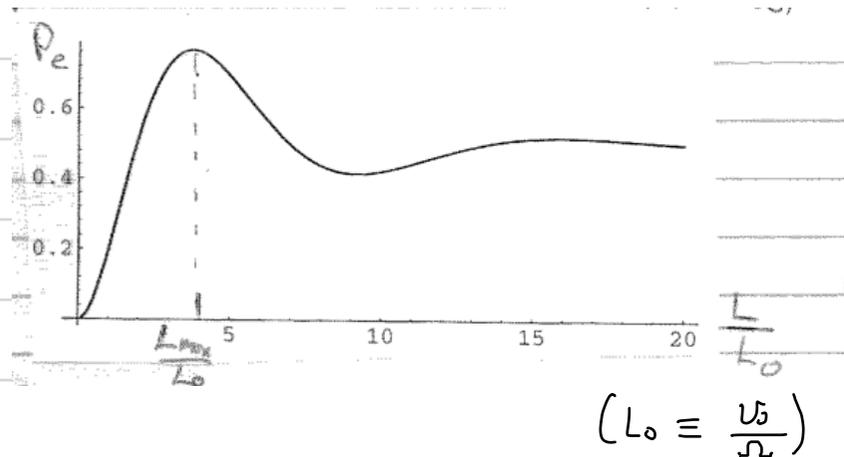
The maximum  $P_{\uparrow}$  occurs at  $L_{\max} = 3.77 L_0 \approx 1.20\pi \frac{v_0}{\Omega}$ . We can understand this from the fact that the most probable speed is  $1.2v_0$
