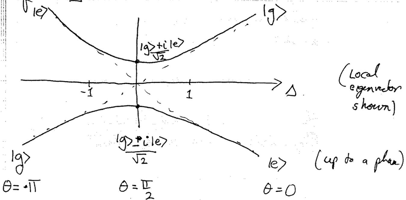
According to the adiabatic theorem of quantum mechanics, for a time dependent Hamiltonian that varies slowly, if we start in an eigenstate we stay in the local eigenstate. Thus according to the curve above, we we adiabatically follow the lower branch, so that the state evolve from  $|g\rangle \rightarrow \frac{1}{\sqrt{2}}(|g\rangle - i|e\rangle) \rightarrow |e\rangle$
