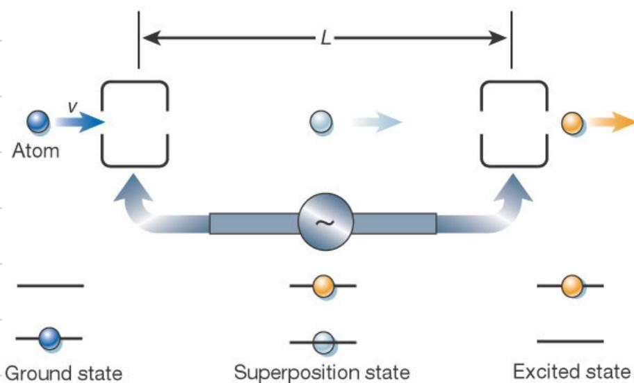
The key idea is to separate two short interaction zones that achieve  $\pi/2$  rotations by a long interaction-free zone. As we will show, the precision with which we can measure  $\omega - \omega_0$  is set by  $L$ , which can be made much longer than for the single zone case.
