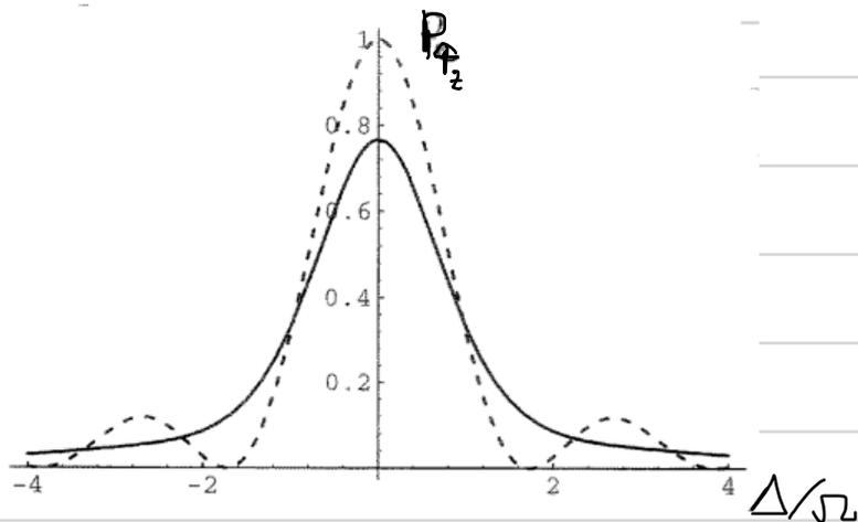
For reference, I have added the curve for mono-energetic spins (dashed curve). We see that the spread in speeds leads to a broadening of the resonance lineshape.
