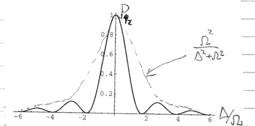
The linewidth of this curve determines the uncertainty of the resonance frequency. For the Rabi method,  $\delta(\omega - \omega_0) \sim \frac{1}{\Omega} = \frac{\pi}{T}$ . This is just an expression of the Fourier time - frequency uncertainty principle.
