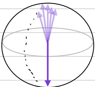
Distribution of speeds  $\rightarrow$  Distribution of interaction times  $\rightarrow$  Distribution of rotation angles on the Bloch sphere.
