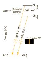
These two lines are known as the "sodium doublet". The transition  $3s_{1/2} \rightarrow 3p_{1/2}$  is known as "D1" and  $3s_{1/2} \rightarrow 3p_{3/2}$  known as "D2". All the alkalis have this basic structure.
