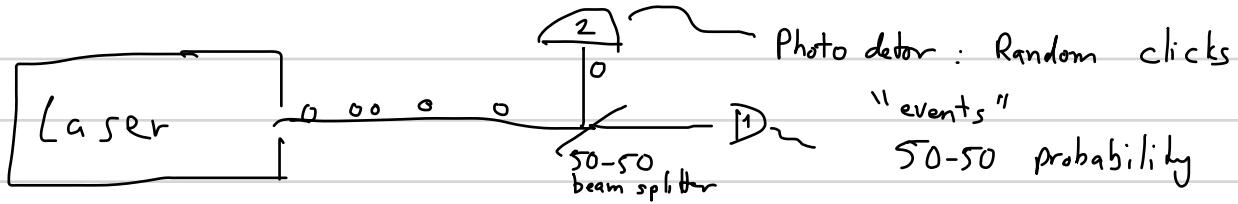
As we will see, the field of the laser can be understood as a stream of photons emitted at random times. Each photon has a probability of being reflected and transmitted at the beam splitter. Whereas the classical intensity is always divided, the photons are quantum that are indivisible; either detector-1 or detector-2 clicks.
