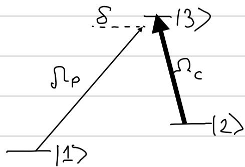
We drive the  $|2\rangle \leftrightarrow |3\rangle$  transition with a strong "coupling laser," Rabi frequency  $\Omega_c$ . The transition  $|1\rangle \leftrightarrow |3\rangle$  is driven with a weak "probe laser," Rabi frequency  $\Omega_p \ll \Omega_c$ .
