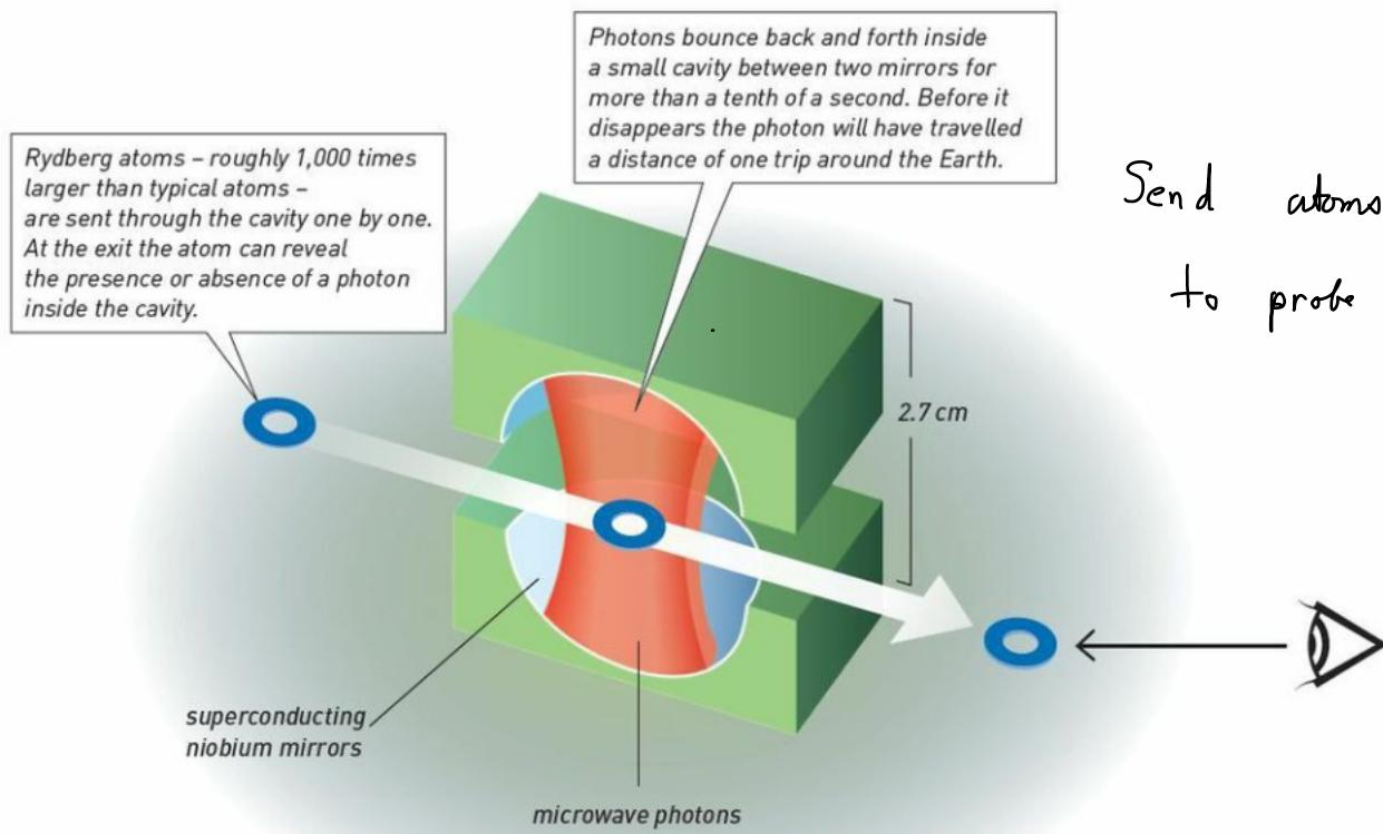
Haroche cavity: Best mirrors ever produced. Photon lifetime in cavity  $T_{\text{cav}} = 0.13 \text{ seconds}$ .
