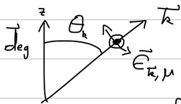
$\Rightarrow \sum_{\mu} |\vec{d}_{eg} \cdot \vec{E}_{\vec{k},\mu}|^2 = \sin^2\theta_k |\vec{d}_{eg}|^2$  (dipole emission pattern)
