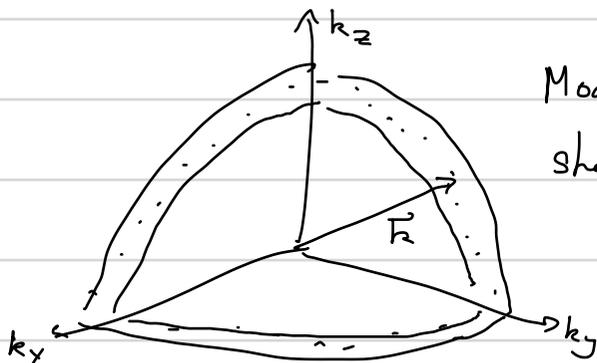
Mode density in a spherical shell in  $k$ -space:  $\omega_k^2$  dependence from 3D space
