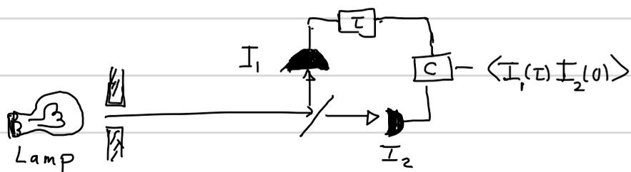
Two detectors are placed symmetrically on either side of a 50-50 beam-splitter. The signal from detector-1 is correlated with detector-2 after a delay  $\tau$ . The result is the correlation between the intensity of the field entering the beam-splitter at two different times. Again, any photon will either be transmitted or reflected, but the correlation is not due to the interference of two paths that any individual photons. Nonetheless, HBT measured the following signal
