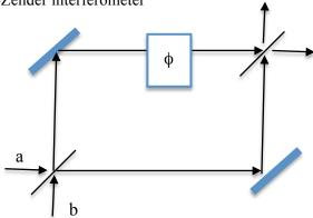
The 50-50 beam splitters are thin black lines and the mirrors are thick blue lines. We assume here that the optical path lengths of the two arms of the interferometer are equal. A phase shifter  $\phi$  is placed in the upper arm.
