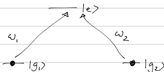
Two possible "paths" to absorption. There exists a superposition  $|\psi_{\text{dark}}\rangle = \alpha_1 |g_1\rangle + \alpha_2 |g_2\rangle$ , such that these two paths destructively interfere.
