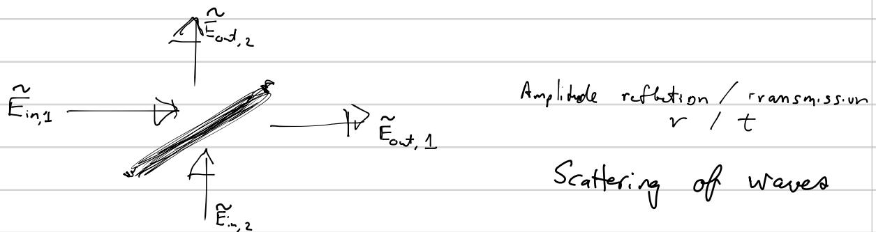
$$\begin{bmatrix} \tilde{E}_{\text{out},1} \\ \tilde{E}_{\text{out},2} \end{bmatrix} = \begin{bmatrix} t & r \\ r & t \end{bmatrix} \begin{bmatrix} \tilde{E}_{\text{in},1} \\ \tilde{E}_{\text{in},2} \end{bmatrix} \Rightarrow \begin{aligned} \tilde{E}_{\text{out},1} &= t \tilde{E}_{\text{in},1} + r \tilde{E}_{\text{in},2} \\ \tilde{E}_{\text{out},2} &= r \tilde{E}_{\text{in},1} + t \tilde{E}_{\text{in},2} \end{aligned}$$
