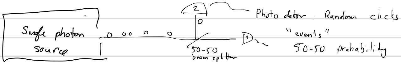
Let us consider a quantum optical source which delivers a stream of individual photons. Each photon has a probability of being reflected and transmitted at the beam splitter. Whereas the classical intensity is always divided, the photons are quantum that are indivisible, either detector-1 or detector-2 clicks.
