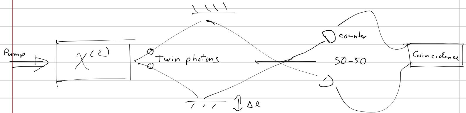
Pairs of identical (twin) photons are incident on a 50-50 beam splitter
