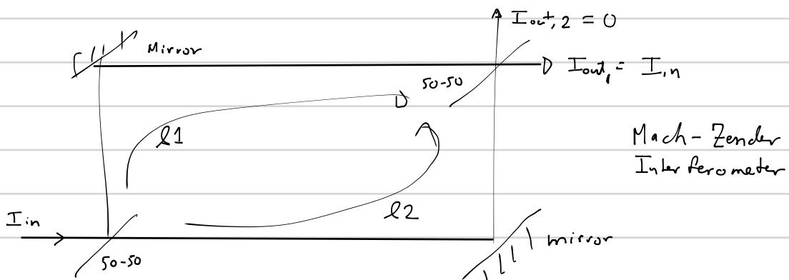
As long as the two paths  $l_1$  and  $l_2$  are equal, all of the intensity exits port-1 of the second 50-50 beam splitter, and no intensity exist port 2! This, of course is interference - the two alternative paths are said to interfere such that there is constructive interference for the beam to emerge port-1 and complete destructive interference for emerging port-2.
