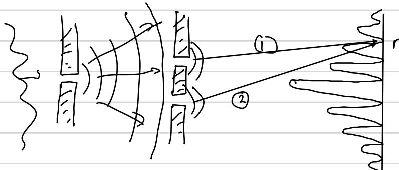
Interference of electric field  $E(r) = E_1 + E_2 \Rightarrow$  Intensity  $I(r) \propto (E_1 + E_2)^2$
