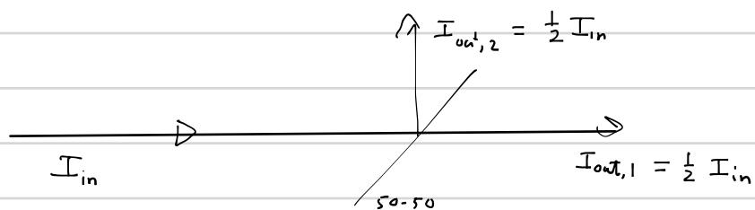
50-50 means 50% of the intensity is transmitted and 50% is reflected. Of course, the same would be true if the input field were incident in the other input port.
