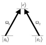
The two ground states are resonantly coupled to the excited state, each with a different Rabi frequency. Taking the two ground states as the zero of energy, then in the RWA (and in the rotating frame) the Hamiltonian is
