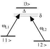
Levels  $|1\rangle$  and  $|2\rangle$  are connected to level  $|3\rangle$  on two dipole-allowed transitions driven by lasers at frequencies  $\omega_{L1}$  and  $\omega_{L2}$  respectively. Laser-1 is detuned from resonance by  $\Delta$ . Difference between the detunings of lasers 1 and 2 is  $\delta = (\omega_{L1} - \omega_{L2}) - (E_2 - E_1)/\hbar$ .
