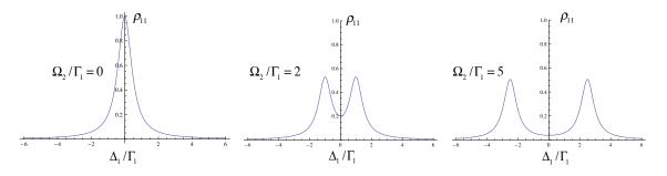
For no coupling, we see the familiar Lorentzian lineshape. As the coupling increases so that  $\Omega_2 > \Gamma_1$ , we see the line split into a doublet known as the Autler-Townes splitting.
