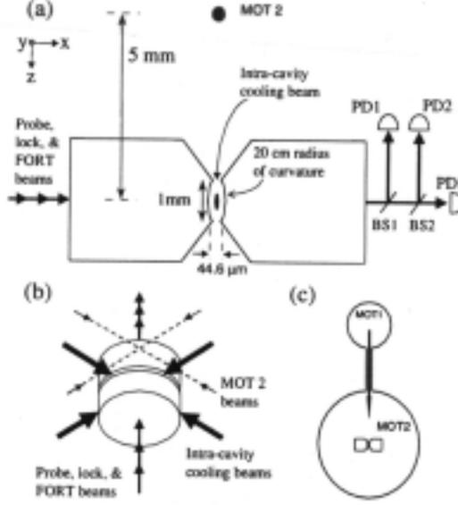
Fig. 5. Schematic of the experimental apparatus. (a) The dichroic beam splitter BS1 sends the cavity-length-stabilizing beam to PD1. BS2 separates the FORT (sent to PD2 for locking) and cavity QED beams (sent to PD3 for balanced heterodyne detection). (b) Beam geometry for intra-cavity cooling and MOT-2. (c) Differentially pumped chamber and two-stage MOT.
