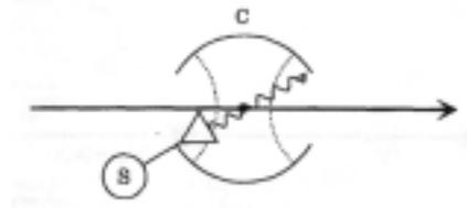
Fig. 7. Scheme of the cavity-QED two bit gate. The control qubit is the state of a superconducting cavity C, either empty or containing one photon. A two-level circular Rydberg atom, slightly detuned from the cavity frequency, carries the controlled bit. The state of the atom is manipulated by a classical field source S. The atom interacts noticeably with S only if the single photon field in C light shifts the transition in resonance with S.
