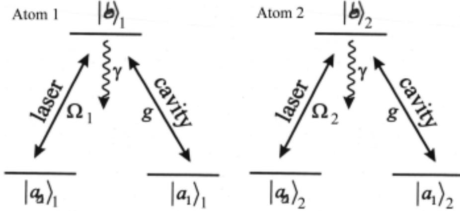
FIG. 3. Two atoms each having a three-level system are coupled to the same cavity, but different laser beams resulting in two Rabi frequencies  $\Omega_1$  and  $\Omega_2$ .
