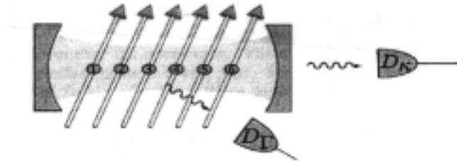
FIG. 1. Realization scheme of a cavity quantum computer using neutral atoms in an optical cavity. The arrows indicate laser beams addressing each atom individually.  $D_R$  and  $D_L$  detect cavity photons and spontaneously emitted photons, respectively.
