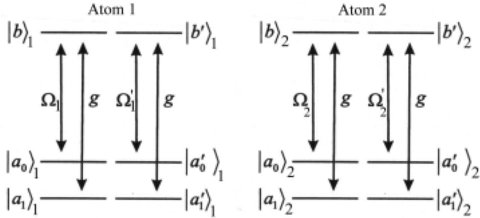
FIG. 4. Two parallel three-level systems in each atom are necessary to perform quantum gates in the cavity QED quantum computer.
