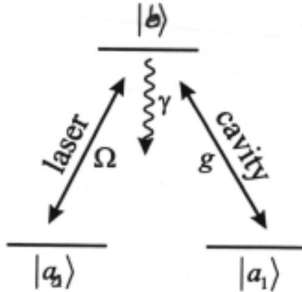
FIG.2. Basic three-level system for the cavity QED quantum computer. One transition is coupled to a laser field; the other is coupled to a quantized cavity mode.
