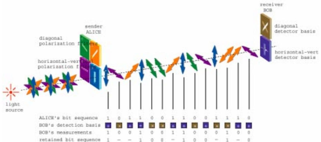
FIG. 1: The BB84 protocol by Bennet and Brassard ([4]) using horizontal, vertical,  $-45^\circ$  and  $+45^\circ$  polarisations. (Figure from [10])
