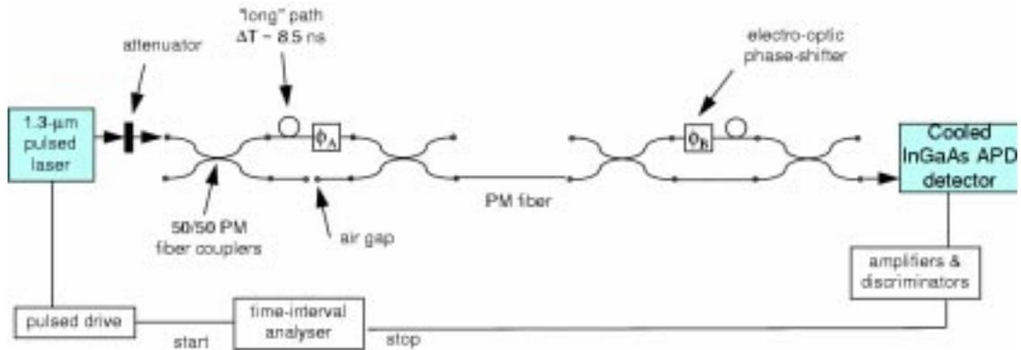
FIG. 3: Schematic representation of the optical system for the Los Alamos QKD prototype, Figure from [11]
