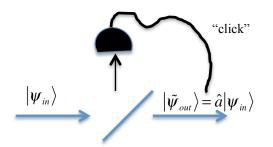
The light is incident on a highly transmitting beam splitter. Rarely one photon is reflected and detected. Conditioned on that "click," the output state has one of the photons annihilated. This state is "post selected" and the probability of producing it is rare. Nonetheless, this is a highly non-Gaussian operation.
