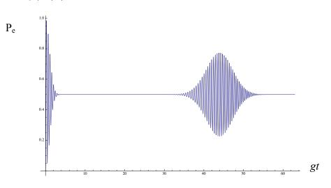
The collapse is due to the variation of the quantum Rabi oscillations with different number; the revival is uniquely a quantum effect arising from the discreteness of the quantized field, occurring at a time  $gt_r \approx 2\pi \sqrt{\langle n \rangle}$  for large  $\langle n \rangle$ .
