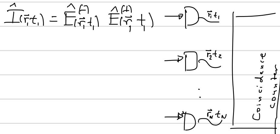
$$P_{\text{coincidence}} \propto \langle : \hat{I}(\vec{r}_1, t_1) \hat{I}(\vec{r}_2, t_2) \cdots \hat{I}(\vec{r}_N, t_N) : \rangle^{\text{Normal ordering}}$$
