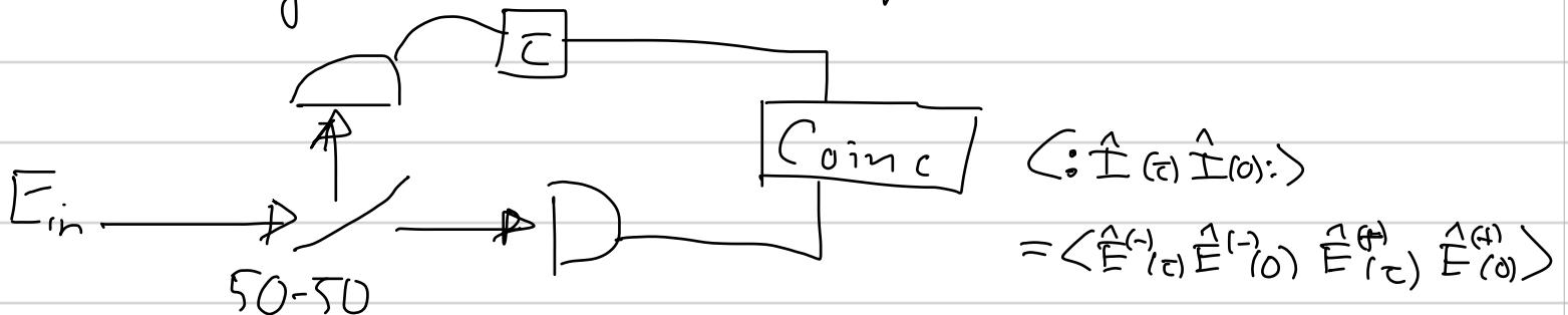
Photons counters, symmetrically placed on opposite output ports of a 50-50 beam splitter
