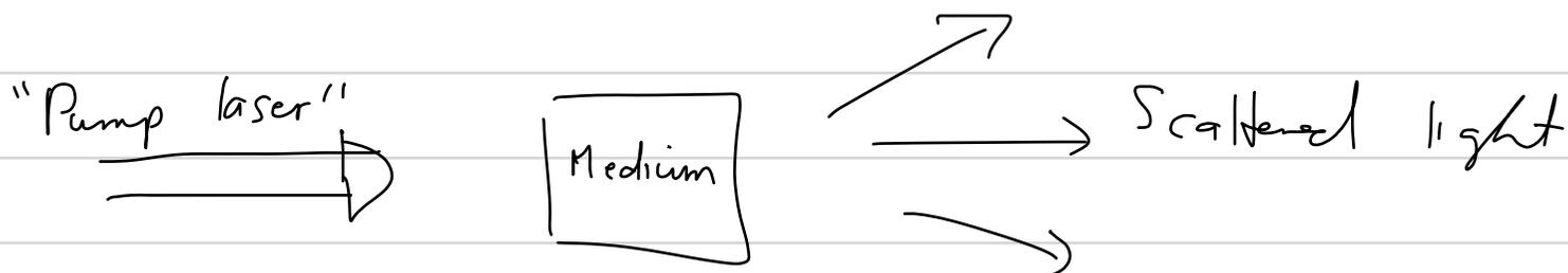
In this picture, the medium mediates interactions between modes of the electromagnetic field. In steady-state, the medium's polarization density is determined by the field. In a perturbative regime, we can expand in power series in the field amplitude
