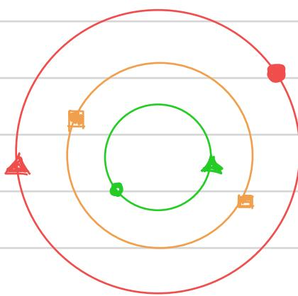
Circles, Squares, and triangles represent different conjugate pairs. Typically apertures are used at the output face to filter out a subset of the possible processes.
