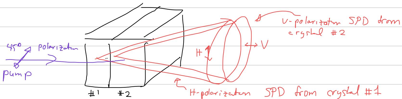
The crystals are oriented such that type-I SPD occurs in each crystal with H-polarization downconverted photons produced in #1 when the pump is V-polarized and V-polarized downconverted photons produced in #2 when the pump is H-polarized. By orienting the pump at 45°, and for crystals thin enough the two possible down conversion processes are indistinguishable.
