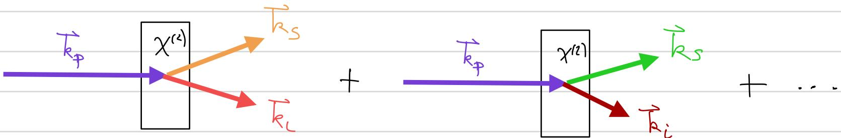
The pattern of spontaneously emitted photon pairs depends on the phase matching condition  $\omega_p = \omega_i + \omega_s$ ,  $\vec{k}_p = \vec{k}_s + \vec{k}_i$
