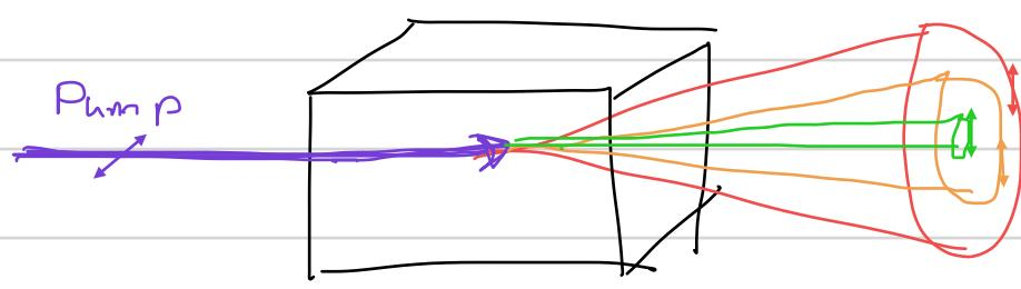
Parametric down conversion rainbow on cones.
