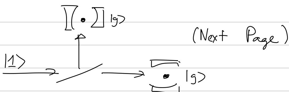
A single photon wave packet is sent to a 50-50 beam splitter. At each output port is an atom cavity in its ground state  $|g\rangle$ . The cavity coupling is such that if a single photon passes through the cavity  $|1\rangle \otimes |g\rangle \rightarrow |0\rangle \otimes |e\rangle$  according to the Jaynes-Cummings interaction.
