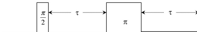
The  $\pi/2$ -pulse about the x-axis to bring all spins onto the y-axis of the Bloch sphere. For a time  $\tau$ , the spins randomly precess about the z-axis and the ensemble dephases. The  $\pi$ -pulse about the x-axis acts to time reverse the process. An “echo” signal will be seen at a time  $\tau$  later when the spins “refocus” and returns to its initial. **Explain this process using this Bloch sphere.**
