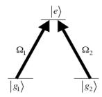
The two ground states are resonantly coupled to the excited state, each with a different
