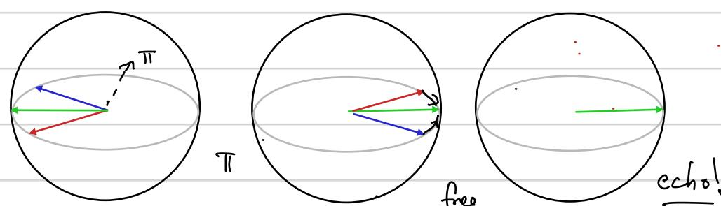
The  $\pi$ -pulse flips the spins so that the spins refocus at time  $\tau$
