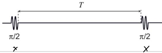
We seek the probability  $P_0 = \langle 0 | \hat{\rho}_{\text{out}} | 0 \rangle$  where  $\hat{\rho}_{\text{out}}$  is the output state of the "interferometer." Without decoherence,  $\hat{\rho}_{\text{out}} = \hat{U}_x^{(\frac{T}{2})} \hat{U}_z^{(\Delta t)} \hat{U}_x^{(\frac{T}{2})} | 1 \rangle \langle 1 | \hat{U}_x^{(\frac{T}{2})} \hat{U}_z^{(\Delta t)} \hat{U}_x^{(\frac{T}{2})}$
