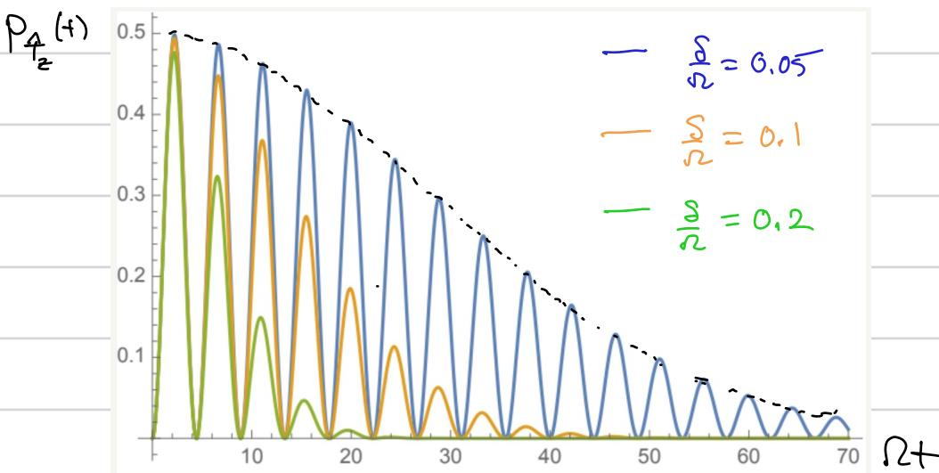
We see here the dephasing of the oscillations with a Gaussian envelope due to the Gaussian spread in detunings
